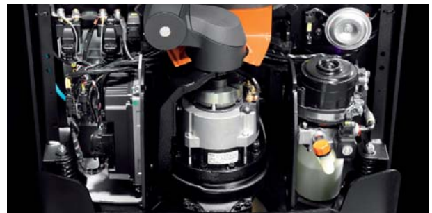
The fixed motor has no moving cables
